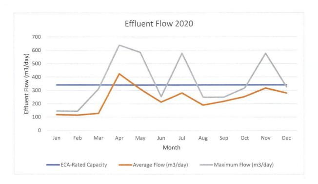
The Latchford Sewage Treatment System operated within its required capacity throughout 2020. Compliance is achieved when the annual average daily flow does not exceed 341  $\text{m}^3/\text{day}$ . The average daily flow for 2020 was 237  $\text{m}^3/\text{day}$  which represents 69.5% of the design capacity. The maximum flow occurred in April when heavy precipitation and snow melt contributed to a maximum flow of 639  $\text{m}^3/\text{day}$ .
